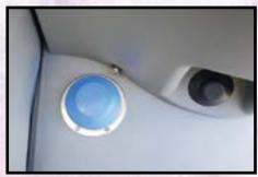
Foot pump provides flushing operation for toilet.
