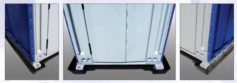
**DESIGN FEATURES:** Thermoformed from tough, impact resistant high molecular weight, high density polyethylene. • Serves as a drip tray to contain water and cleaning solutions during servicing. • Fluids drain towards the rear of the tray to a convenient pump out location. • The trays have a peripheral lip that guides fluids into the pan. • Will fit beneath most portable restrooms. • Support ribs for extra strength beneath the "runners" to raise them out of fluids between servicing.
